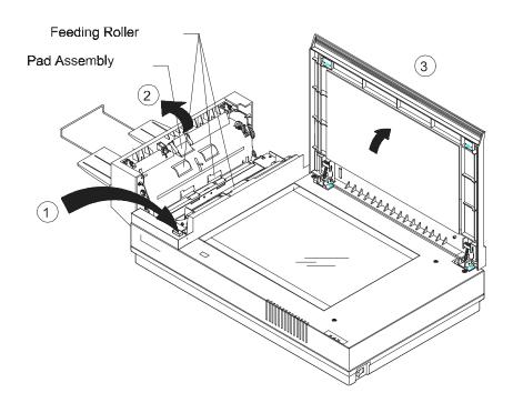
Figure 3-1 Opening the ADF unit and Document Cover
